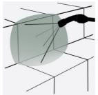
Set the pressure between 0.5 and 1 bar. Apply an even layer to the surface.
